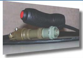
A hand switch, or pickle, also attaches to the lower assembly and is used by the operator to signal when the sighting device is aligned to the chosen aid to navigation. The TBT kit quickly integrates with the charting system, voyage data recorder or any other device that can receive a standard NMEA message.
