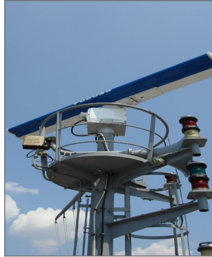
Furuno Radar Installed on USNS Bob Hope
